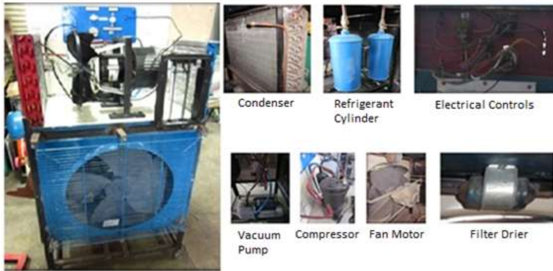
Figure 4. Assembled Innovated Refrigerant Recycling Machine with parts from old air conditioning units
